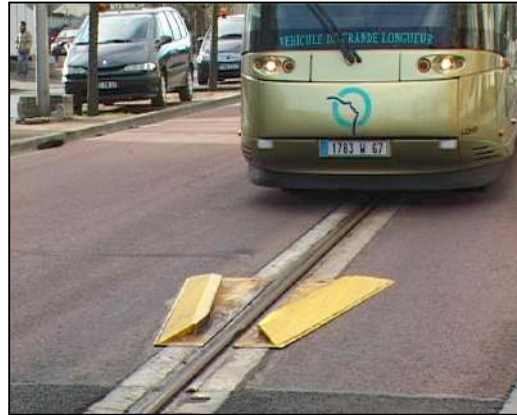
Figure 54: TRANSLOHR SE and the equipment to attach/detach on the rail, the guidance device
