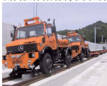
Traction vehicle capable of running on tracks as well as the ground, namely hi-rail car
