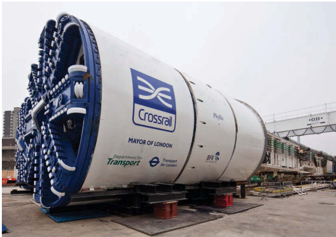
IMAGE 11.5. One of Crossrail's Tunnel Boring Machines, with Back-End Supply of Power, Water, and Concrete Segments
