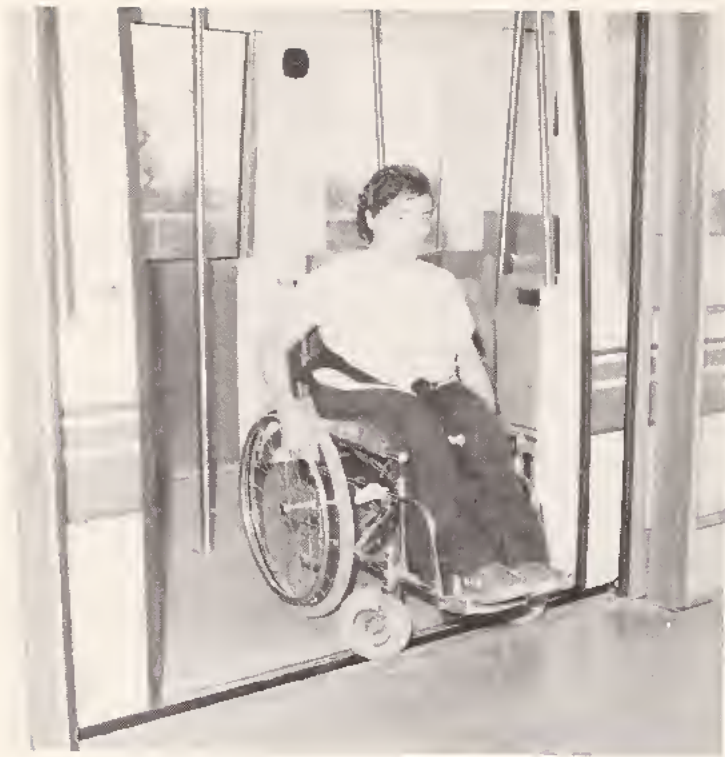
FIGURE 6-1. WHEELCHAIR EGRESS THROUGH DOORS
