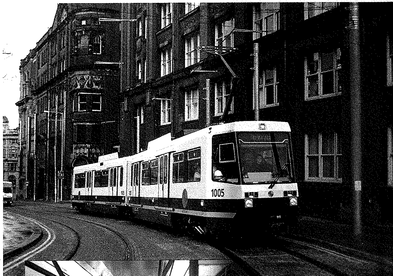
Articulated Light Rail Vehicle Firema type T 68, for the GMA Group - Manchester Metrolink
