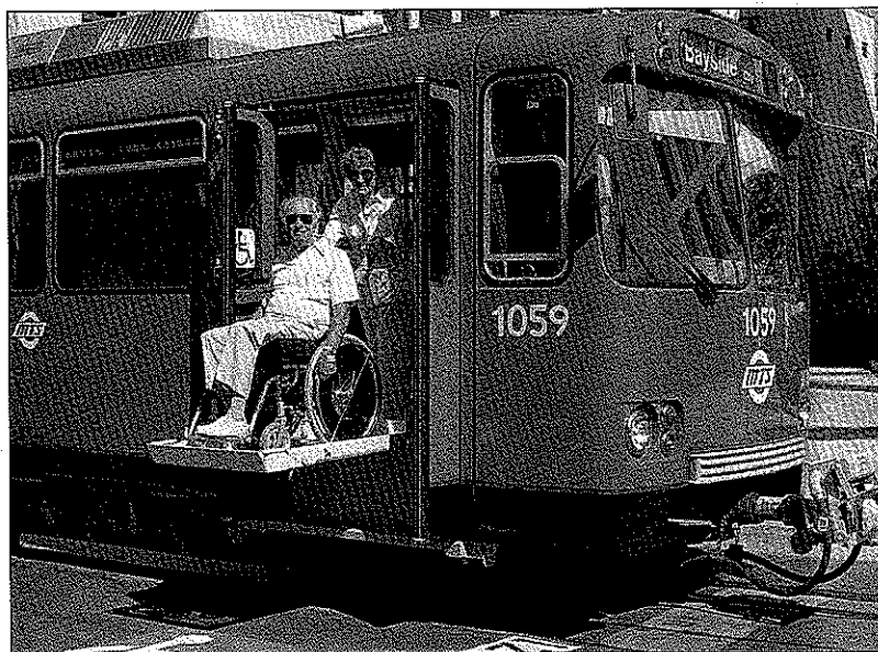
San Diego Trolley has fitted its LRVs with wheelchair lifts, but concern for disabled passengers may see low-floor cars adopted in future schemes
