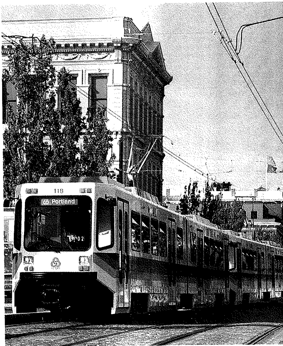
Articulated LRV Nos. 101-126 of the Tri-County Metropolitan Transport District of Oregon/USA (Tri-Met) for the urban mass transit system of Portland. Bi-directional operation with 750 V d.c.
