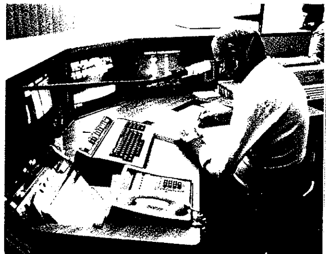
Figure 14. The tram- and bus-operation control system detects every tram and every bus with an accuracy of 10 metres. The computer continuously compares the actual position with the theoretical position and indicates deviations, which can be reacted to with suitable measures - extra vehicles, detours, etc.
