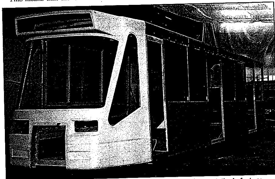
Bodyshell of the new lightweight low-cost LRV at Pullman Transportation's factory.
