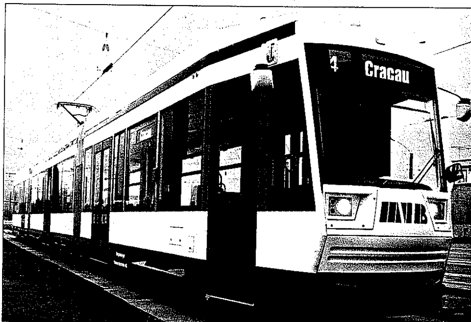
Magdeburg's MGT8D 60% low-floor cars from LHB and ABB have 12 seats standing on 225 mm high boxes, leaving a 675 mm wide corridor
