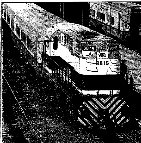
One of three Alco RSD16 diesel-electric locomotives refurbished by TMS.
