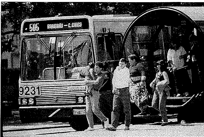
Curitiba's bus system acts much like a typical urban subway system. The conventional bus is modified so that the doors open directly onto an innovative boarding tube station. The floor from bus to boarding tube is level.
