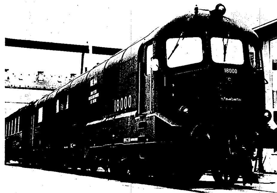
FIG. 12.29. Gas turbine locomotive adapted for adhesion testing.
