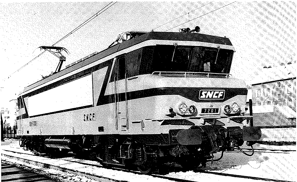
Fig. 19. — BB 7200 class 1,500 V d. c.-4,400 kW electric locomotive, EU 4500 C1 series, designed with dynamically braked monomotor trucks. Maximum speed: 180 km/hr. (112 mph). Maximum speed reverse service: 160 km/hr. (100 mph)
