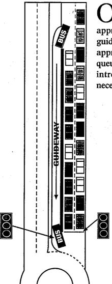
bservers have recorded traffic queue lengths over a period of time on the approach to junctions. The length of the guideway sections has been calculated to be approximately equal to the longest traffic queue. Additional sections of guideway can be introduced in the future if this proves necessary.
