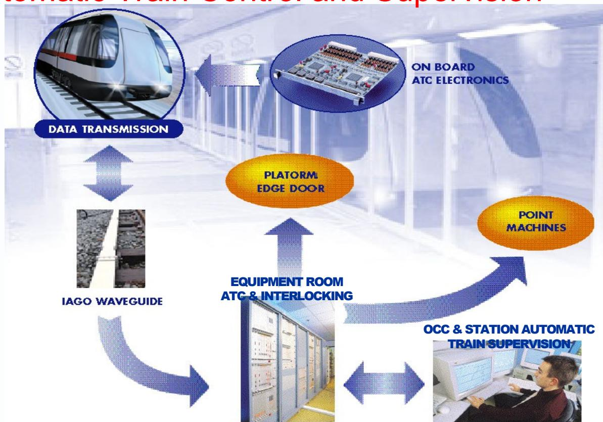
Normal operation : Moving Block with on-board processor
