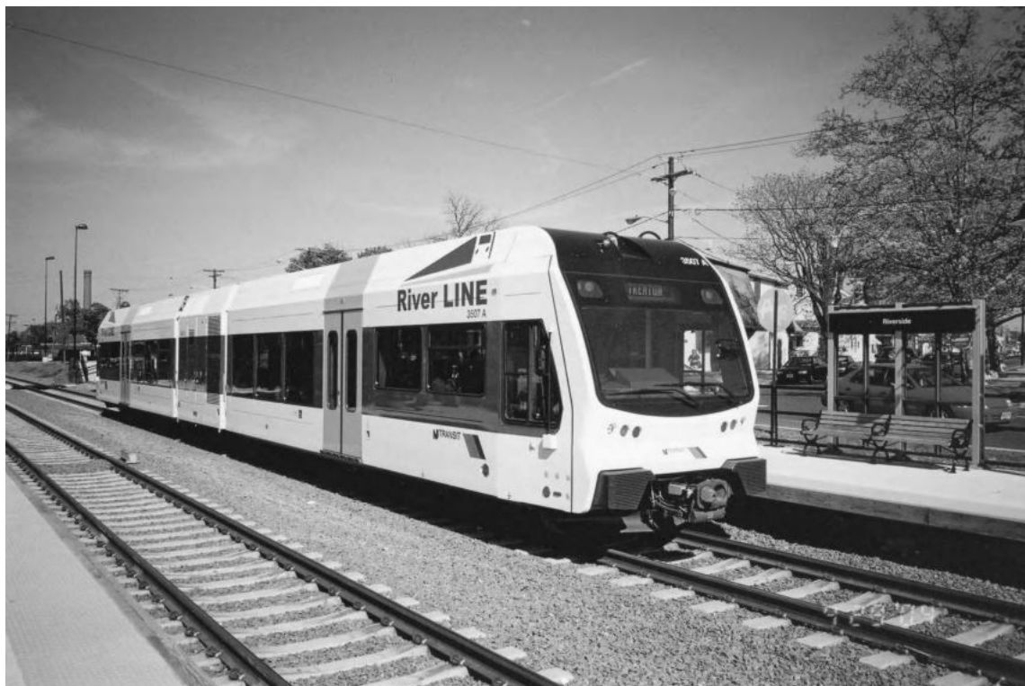
Photo 6.34 Diesel LRT station with medium-height platform in New Jersey (NJ Transit River Line; courtesy of J. W. Vigrass)
