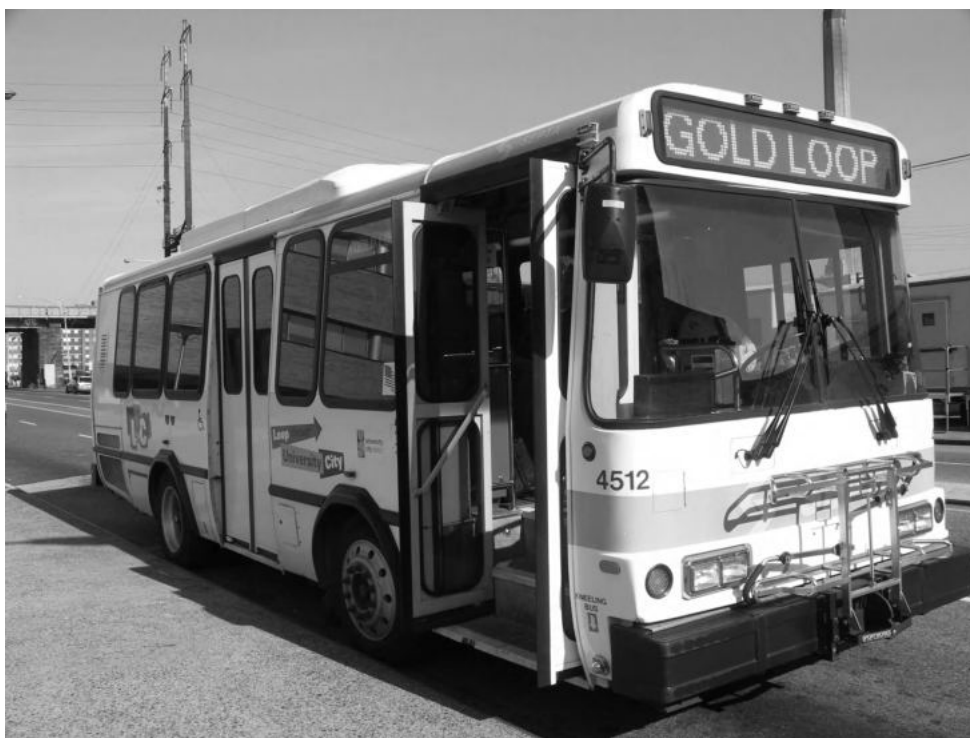
Photo 2.5 Medium-capacity common carrier vehicle (midibus in Philadelphia; courtesy of Karyn J. Cullen)
