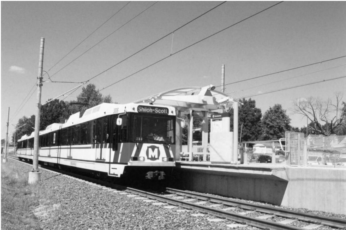
Photo 6.7 Six-axle LRT vehicles at a high-platform station on the Metrolink system in St. Louis
