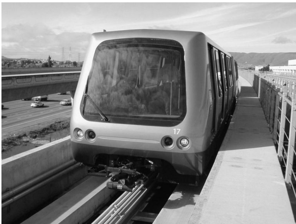
Photo 7.4 Bombardier AirTrain (variant of CX-100 model) AGT vehicle at San Francisco Airport (Courtesy of Bombardier Transportation)
