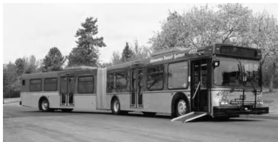
Photo 5.9 Low-floor articulated bus with wheelchair ramp lowered (Courtesy of Edmonton Transit System)
