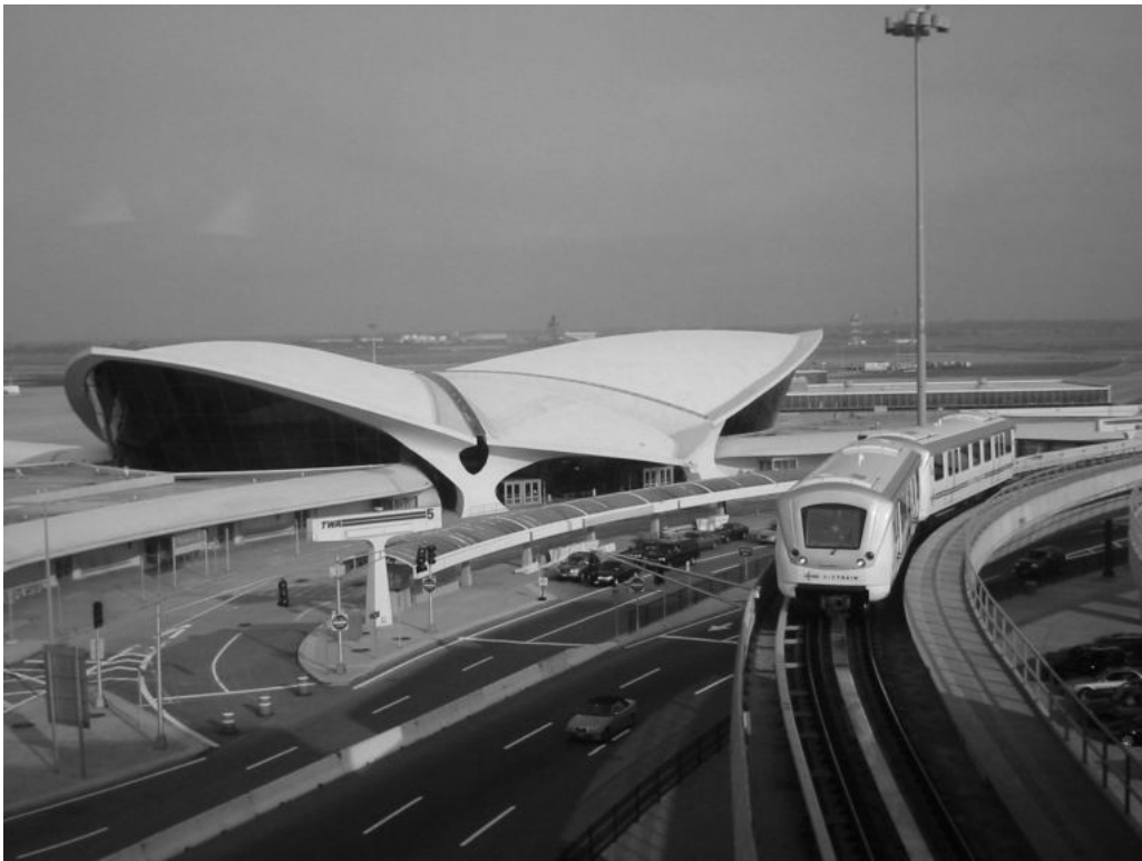
Photo 7.8 UTDC/Bombardier AGT system with LIM propulsion for JFK Airport in New York (© 2004 Hal Dick)
