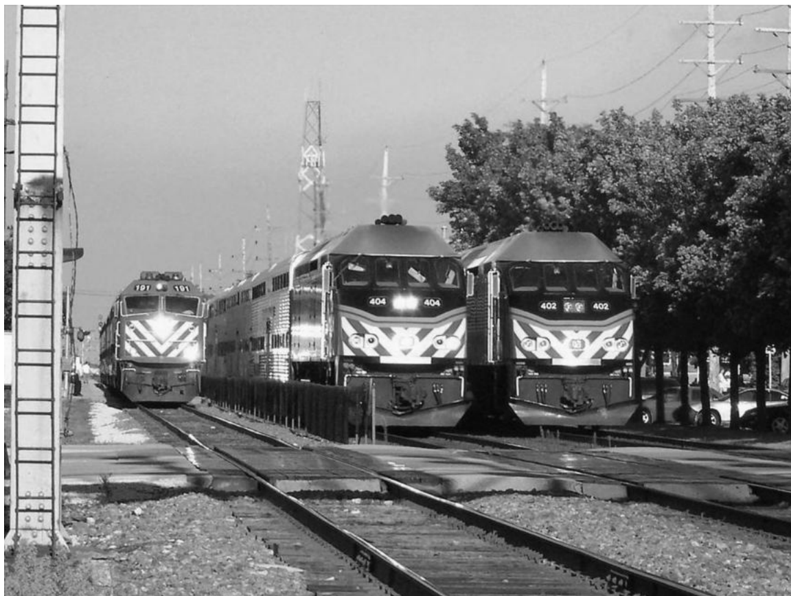
Photo 4.1 Express train (center) bypassing a local train (left) at an off-line station on Chicago's Metra system (Courtesy of Joe LeMay)
