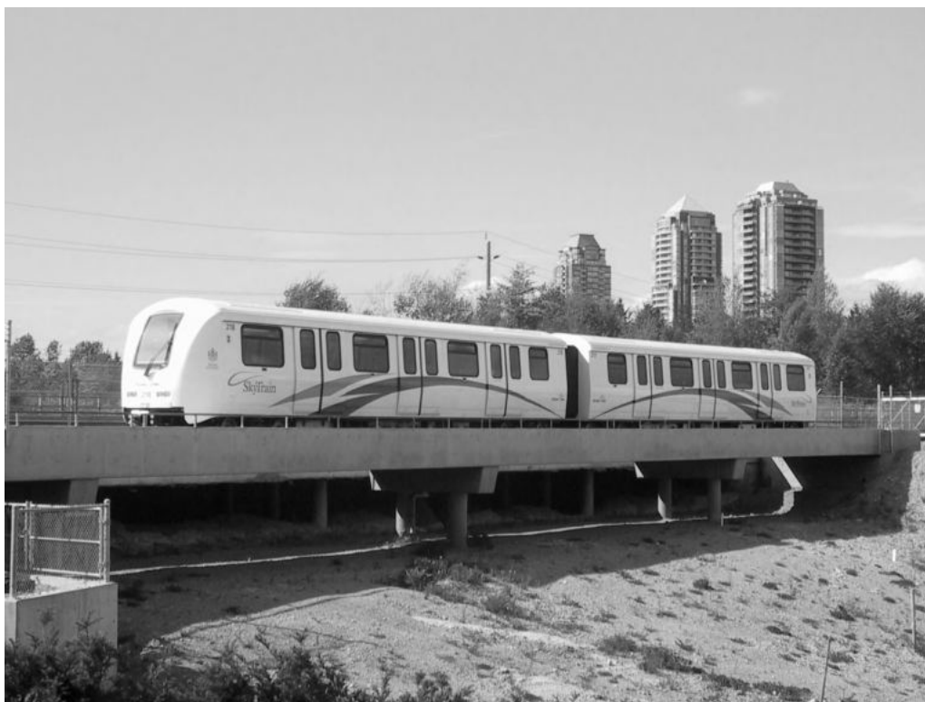
Photo 7.7 Vancouver SkyTrain, high-capacity rail AGT, or a minimetro system (Courtesy of Bombardier Transportation)
