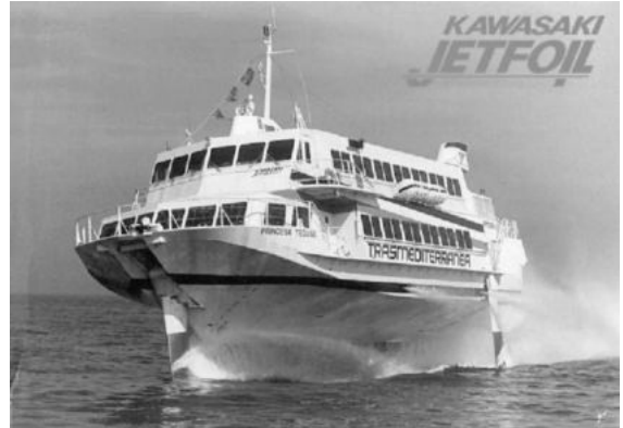
Photo 8.14 High-speed hydrofoil (Courtesy of Kawasaki Heavy Industries, Courtesy of James Aslaksen)
