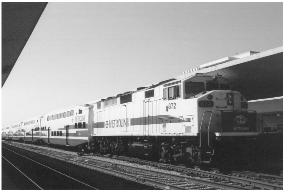
Photo 6.5 Regional rail: Bilevel cars on Los Angeles Metrolink (Courtesy of James R. Greene)
