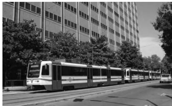
Photo 2.10 A large-capacity vehicle for semirapid transit (LRT in Sacramento; courtesy of Peter Ehrlich)
