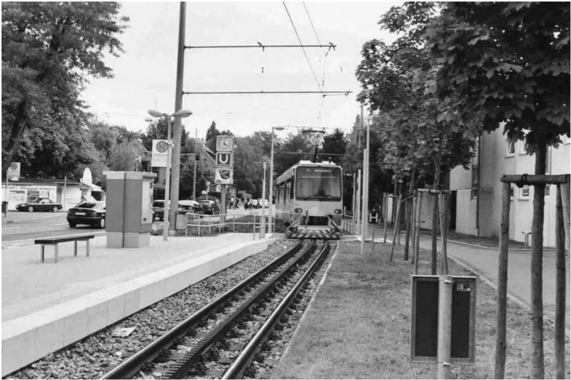
Photo 8.2 Meter-gauge cog railway with bicycle trailer in Stuttgart (Courtesy of Gabriel Tompkins)
