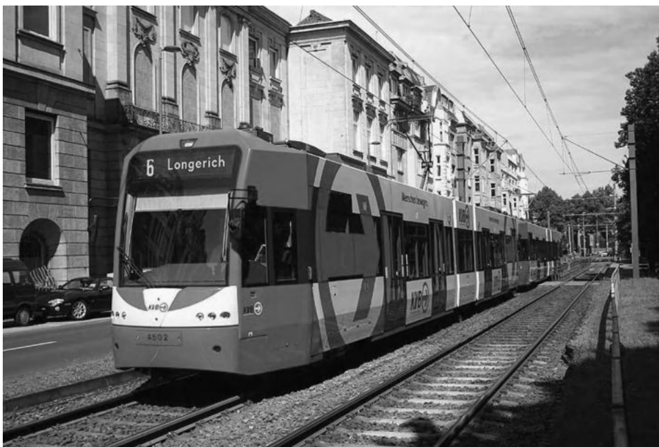
Photo 6.2 LRT: a six-axle low-floor vehicle in Cologne (Siemens K4500; courtesy of Sybic)
