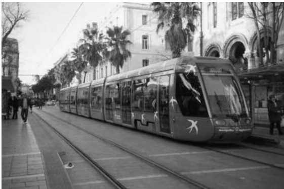
Photo 6.8 Eight-axle LRT vehicle in Montpellier (Courtesy of P. L. Guillemin)
