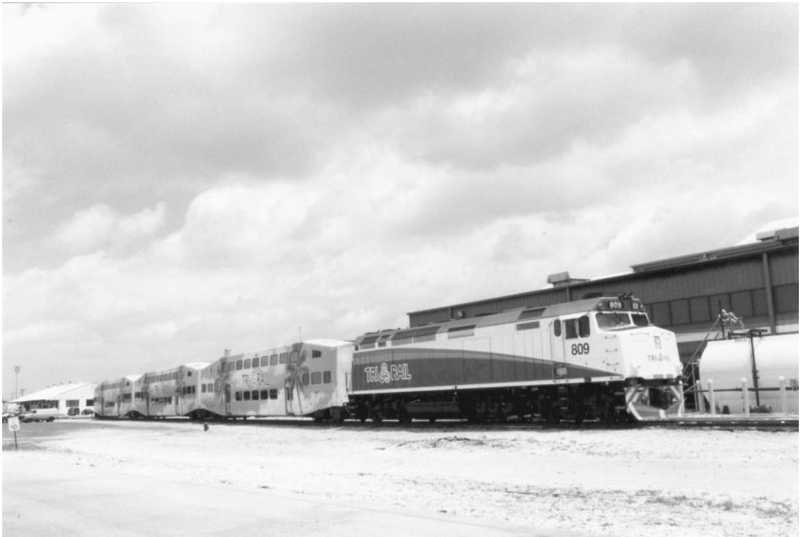
Photo 6.47 Regional rail, with strong trend toward bilevel cars, is being expanded in many large- and medium-sized cities (Courtesy of W. D. Volkmer)
