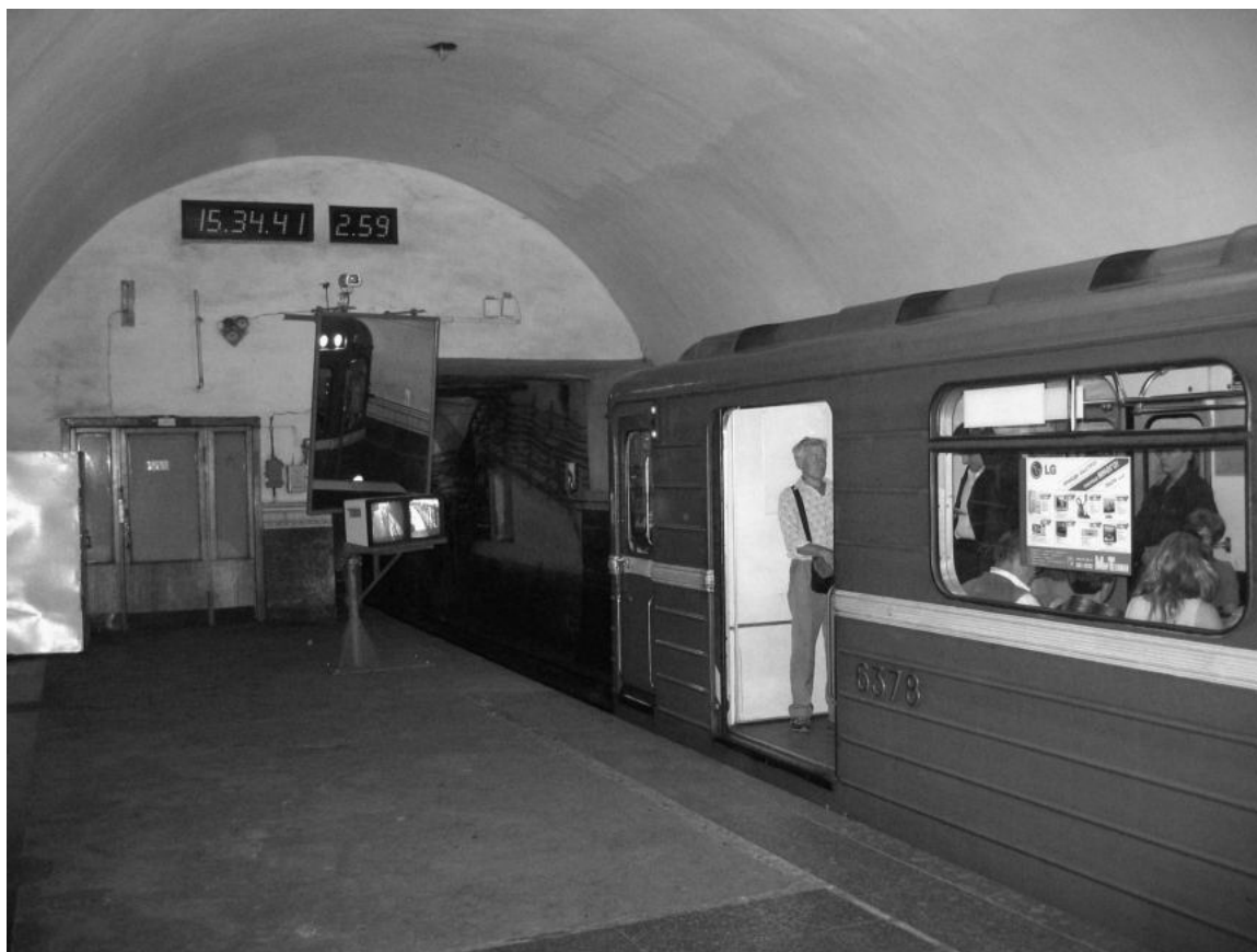
Photo 6.43 Headway clock for maintaining short and reliable headways on Moscow Metro
