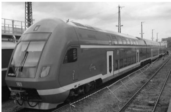
Photo 6.18 Three-car unit bilevel train on Munich S-Bahn (Courtesy of Tobias Köhler)
