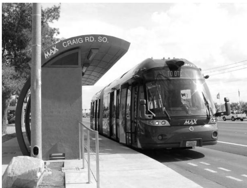
Photo 5.23 BRT in Las Vegas: bus with rail styling. Optical sensor above windshield for automated close docking (Courtesy of NeiTech.)
