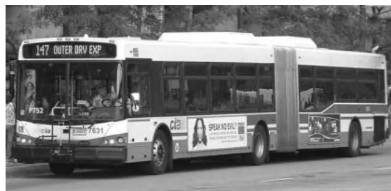
Photo 5.1 A contemporary articulated low-floor diesel bus in Chicago (Courtesy of Kelly Martin)
