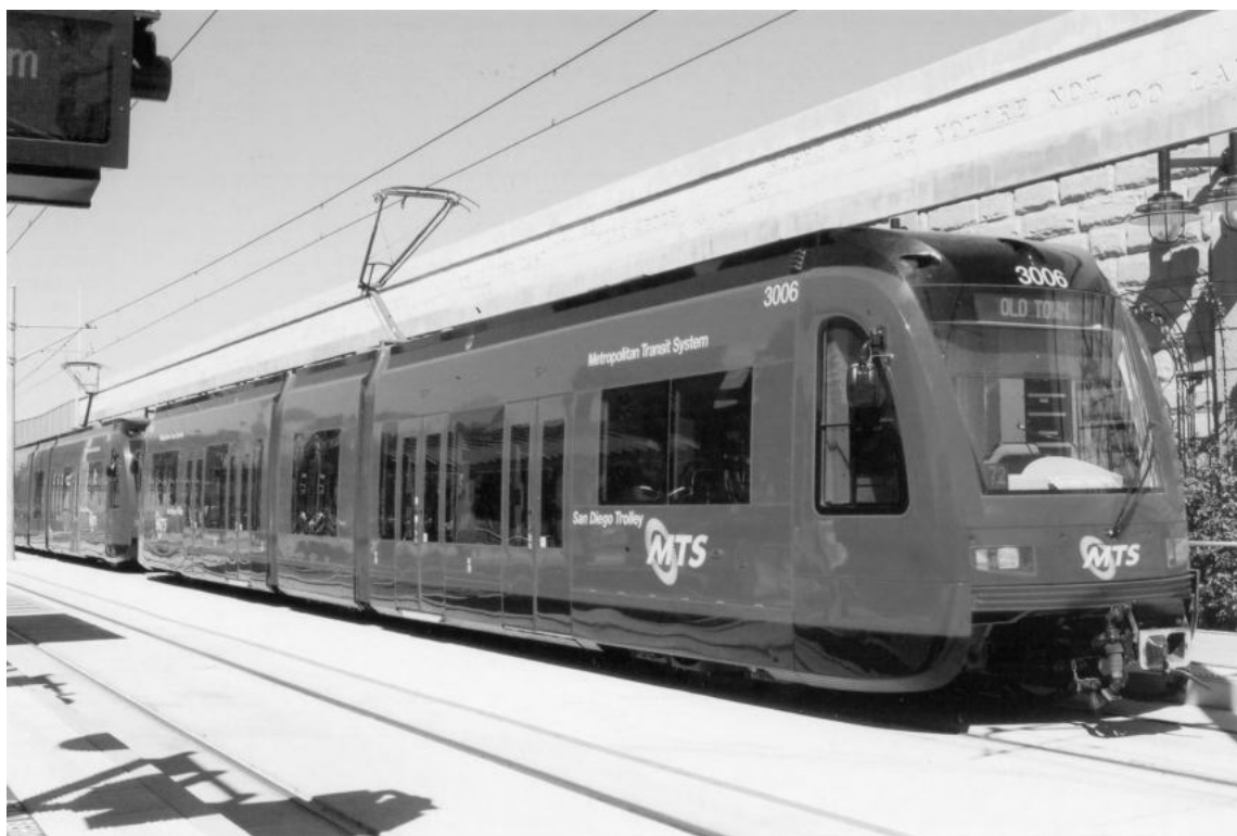
Photo 6.17 Two six-axle LRT train in San Diego (Siemens S70 model)
