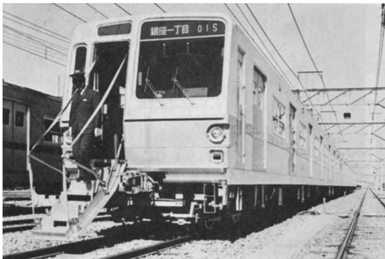
Photo 6.15 Tokyo RRT car with an emergency exit through the front (Courtesy of Teito Rapid Transit Authority)
