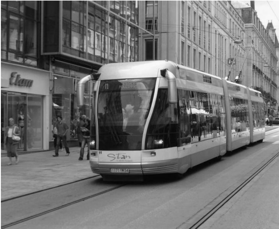
Photo 5.33 Double-articulated trolleybus with guide-rail embedded in street
