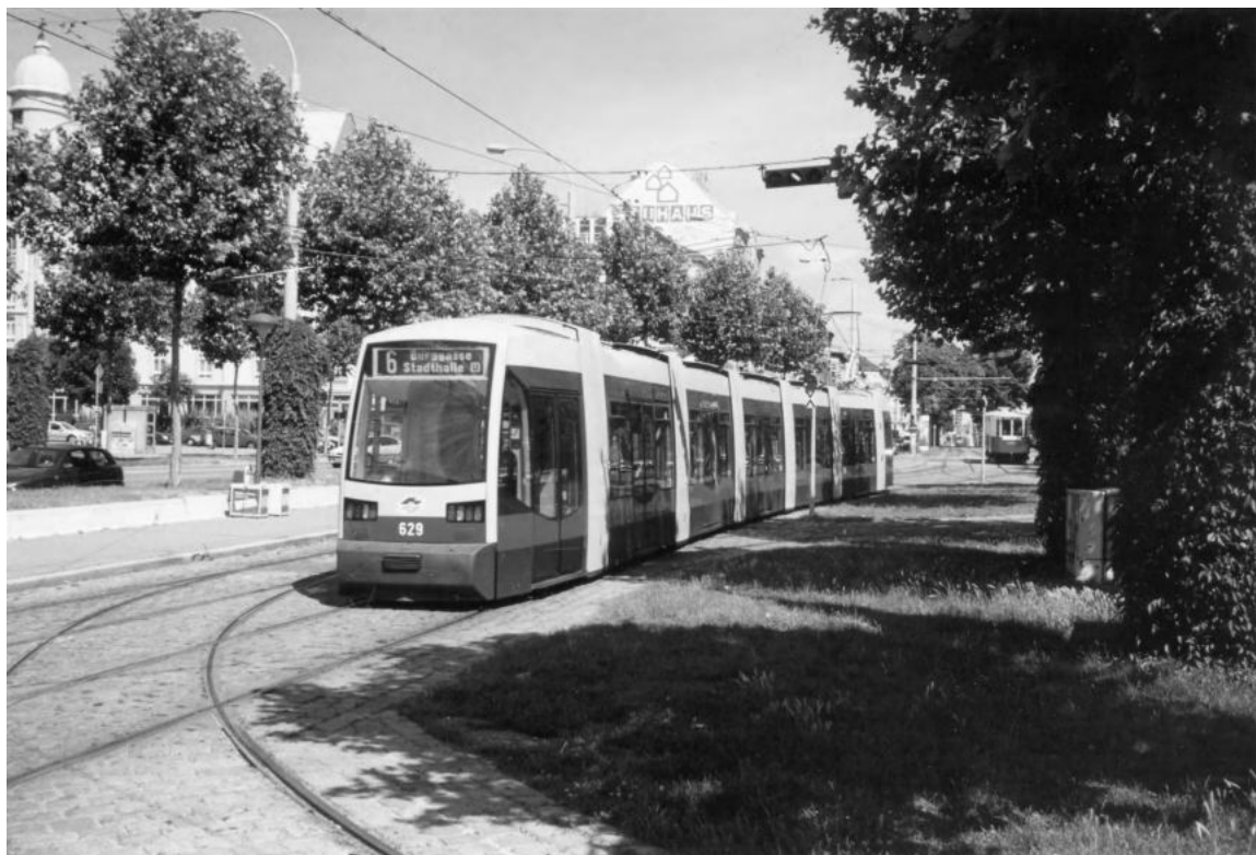
Photo 6.1 A modern streetcar (Siemens Ultra-low-floor model in Vienna)
