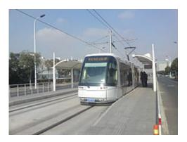
**Zhangjiang Tram** is the only <u>tram</u> line operating in <u>Shanghai</u> today, utilizing a system manufactured by the French <u>Translohr</u> company. It is a <u>rubber-tired tram</u> system, second both in China and Asia.
